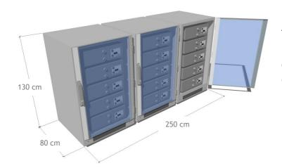
The battery is designed for a minimum 10 years lifetime, it has a total capacity of 67 kWh and can supply a peak discharge power of 730 kW.
